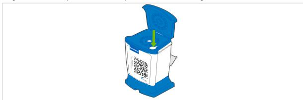
5. Close the cartridge lid and start the test.
